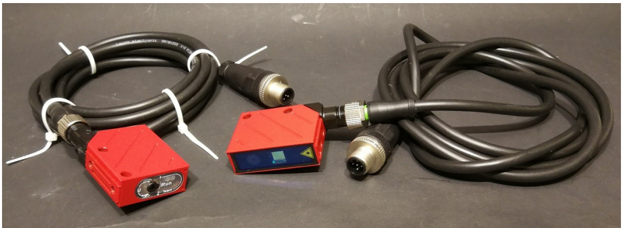
Two identical red Leuze Laser sensor's shown with 1,5 meter wire and M12 connectors.
