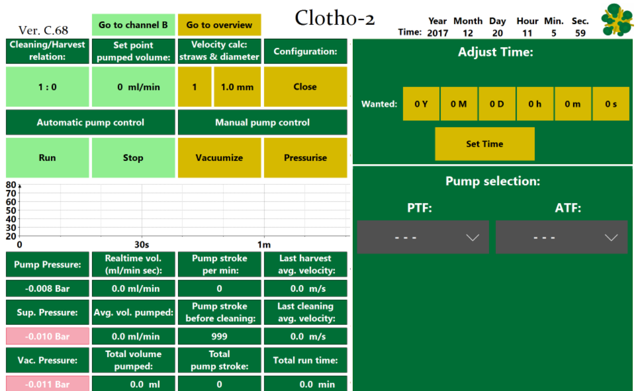
Illustration of the GUI shown on the build-in 5" display with channel A selected.
