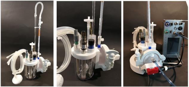
Photos show the size 500 mounted in a Heating-Support-Foot. Red Laser sensor mounted in a Re-Usable-Bracket above the dome of the Thalia-30 Alternating-Single-Use-Exchanger (A-SUE). Clotho Drive Unit from <u>www.perfusecell.com</u> takes care of A-SUE performance.
