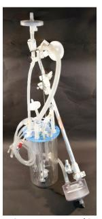
Photos show 3,2 liter SUB integrating HFF and SUB. The red Laser sensor is seen mounted in the white Laser-Support-Clio below the dome of the Clio-100 pump. Of 4 Drive Units from <a href="https://www.perfusecell.com">www.perfusecell.com</a> from bottom: vacuum pump, pressure pump, air reservoir and on top Clotho-1 for single O-SUP control. P-SUB is comfortable mounted on Magnetic-Stirrer-Table (MST) driven by any servo motor.
