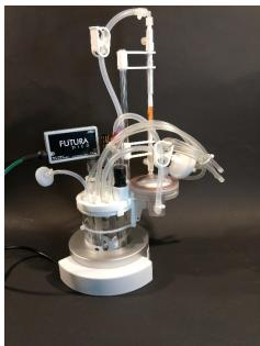
Photos show the mini mounted in a Heating-Support-Foot. Red Laser sensor mounted in a Re-Usable-Bracket above the dome of the Clio-30 pump. Units from <u>www.perfusecell.com</u> include the VisiWell, OneFerm and PICO Futura bio-mass sensor and SUS.
