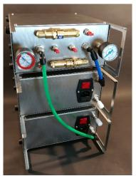
Two Alagonia in Hephaestus U2 Stainless Steel cabinet. Further one Sarpedon reservoir straightening out pulsating and allowing more connections. Sarpedon stacked on top with pressure relief valves and internal hose connections.
